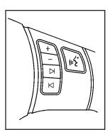
Radio controls are located on the right side of the steering wheel. If your vehicle has this feature, some audio controls can be adjusted at this location.
